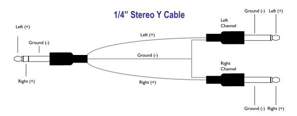
**NOTE:** The I/4" Output must be configured for stereo operation for this type of setup. See "Mono/ Stereo Operation" on page 21 for more information. When connecting directly to a recording device, SCC must be enabled. See "Speaker Cabinet Compensation (SCC)" on page 21 for more information.
